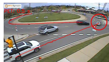
Conflict between motorists exiting and entering roundabout
