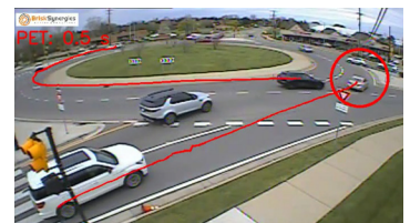
Conflict between motorists exiting and entering roundabout
